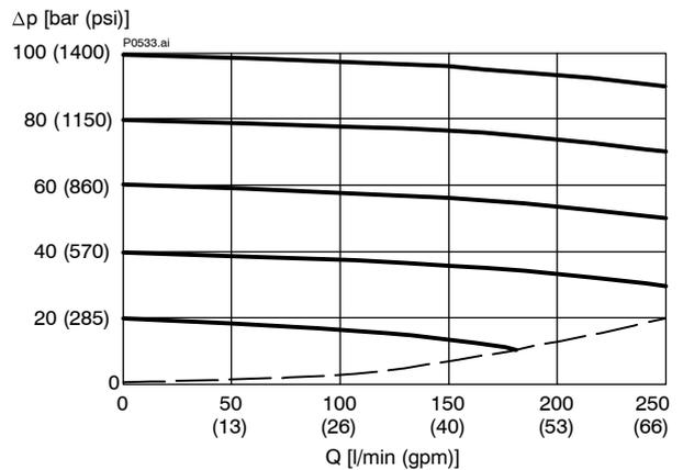
$\Delta p = f(Q)$  Pressure-drop characteristic (40 bar)
