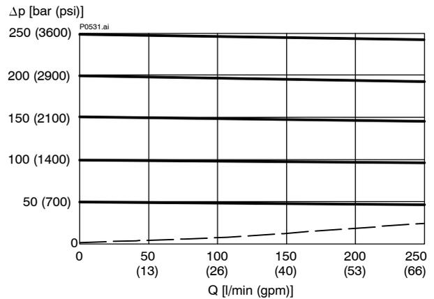
$\Delta p = f(Q)$  Pressure-drop characteristic (160 bar)
