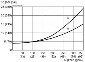
cavity type EB without annular groove
