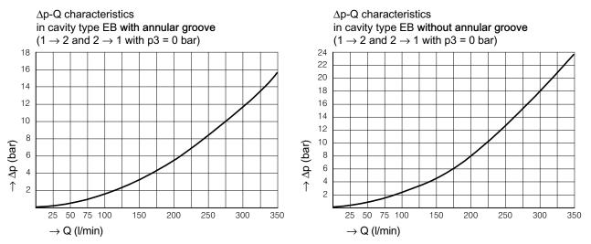
The  $\Delta p$  characteristic is valid when the load pressure in the connection  $1 \rightarrow 2/2 \rightarrow 1$  is greater than the opening pressure. If the load pressure is less than the opening pressure, the load pressure must first rise to overcome the opening pressure before flow can occur.
