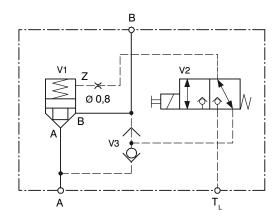
Logic valve application for lowest possible vented pressure with a proportional throttle and bypass compensator
