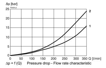
1 = cavity type DJ with annular groove
