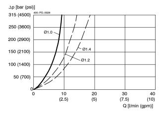
$\varnothing$  1.2 and  $\varnothing$  1.4 orifices drilled out by customer!
