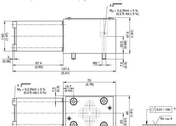
3/3, 4/3, and 4/4 hand operated directional seat valve (double-control model)
