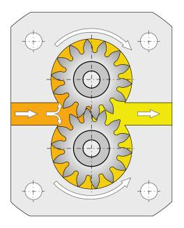
The gears run in a contactless manner in the measuring chamber. The lowfriction bearings or plain bearings act as the bearing elements.
