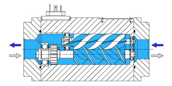
The device is a displacement counter. Two measuring spindles with pitched profile are meshed. They are supported by anti-friction bearings and encased.
