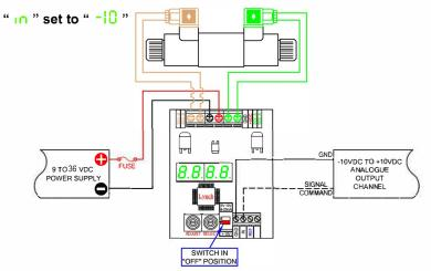
PLEASE NOTE: For "0 to 5 VDC" & "0 to 10 VDC" command input drivers, it is recommended to use independent negative conductors for power supply and analogue output channel (PLC/PC) to maintain command signal accuracy due to voltage drop on long cable runs.
