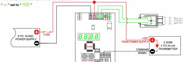
PLEASE NOTE: For "0 to 5 VDC" & "0 to 10 VDC" command input drivers, it is recommended to use independent negative conductors for power supply and analogue output channel (PLC/PC) to maintain command signal accuracy due to voltage drop on long cable runs.
