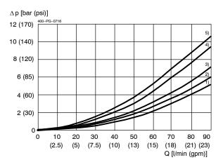
$\Delta p = f(Q)$  Pressure drop - Flow rate characteristic Spool types: A / B, D, G, and H
