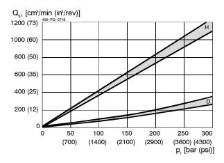
Q<sub>ST</sub> = Pilot-oil consumption Spool types: A / B and G
