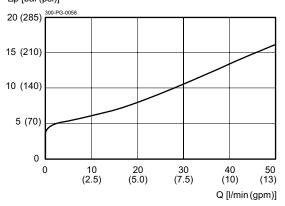
Lifting function, flow direction A to B
