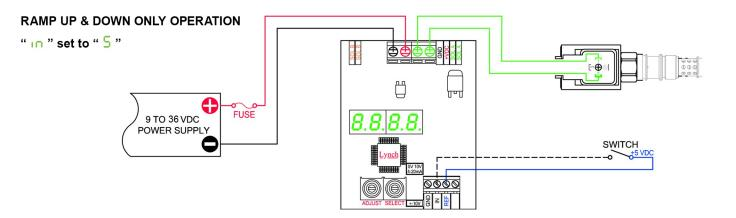
**PLEASE NOTE:** For "0 to 5 VDC" & "0 to 10 VDC" command input drivers, it is recommended to use independent negative conductors for power supply and analogue output channel (PLC/PC) to maintain command signal accuracy due to voltage drop on long cable runs.
