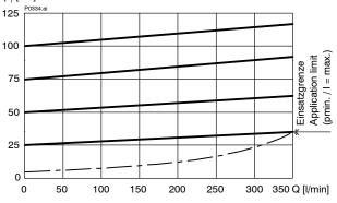
p = f(Q) Pressure - Flow rate characteristic  $p_N = 160$  bar  $p_1$  [bar]
