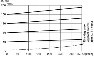
p = f(Q) Pressure - Flow rate characteristic  $p_N = 250$  bar  $p_1$  [bar]
