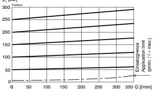
p = f(Q) Pressure - Flow rate characteristic  $p_N = 350$  bar  $p_1$  [bar]
