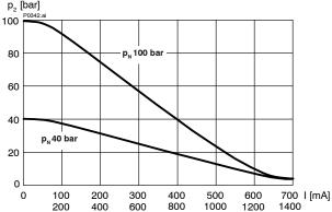
p = f(I) Pressure adjustment characteristic (Q = 10 I/min)  $p_2$  [bar]
