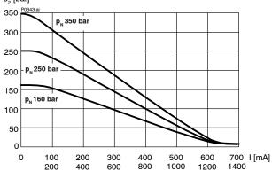
p = f(Q) Pressure - Flow rate characteristic  $p_N = 40$  bar p, [bar]
