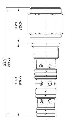
Version "S": Einstellschraube (*Standard*) Version "S": adjustment screw (*standard*)
