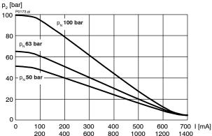
p = f (Q) Pressure - Flow rate characteristic  $p_N$  = 50 bar  $p_2$  [bar]
