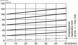
p = f(Q) Pressure - Flow rate characteristic  $p_N = 230$  bar  $p_p[bar]$
