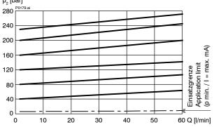
p = f (I) Pressure adjustment characteristic (Q = 5 I/min)
