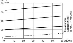
p = f(Q) Pressure - Flow rate characteristic  $p_N = 160$  bar p. [bar]
