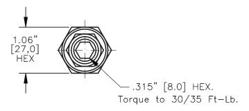
Turn screw clockwise to increase the pressure setting.
